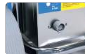
Water mains connection
