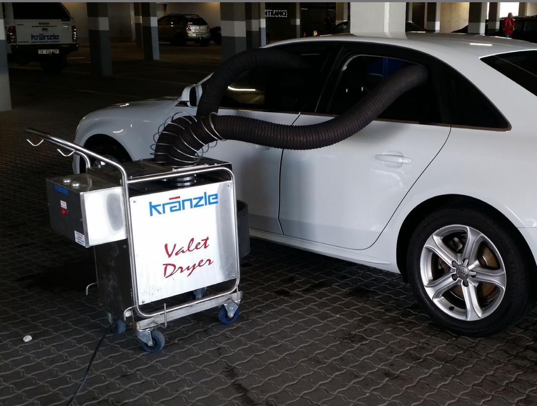
Once a vehicle has been through the valet process, time and during winter may not allow the outside ambient temperature to dry the interior of the vehicle quickly enough. For this purpose we supply a valet dryer that consists of a blower, heater and two hoses that are inserted through the car windows. This heating of the interior greatly reduces the drying period.
